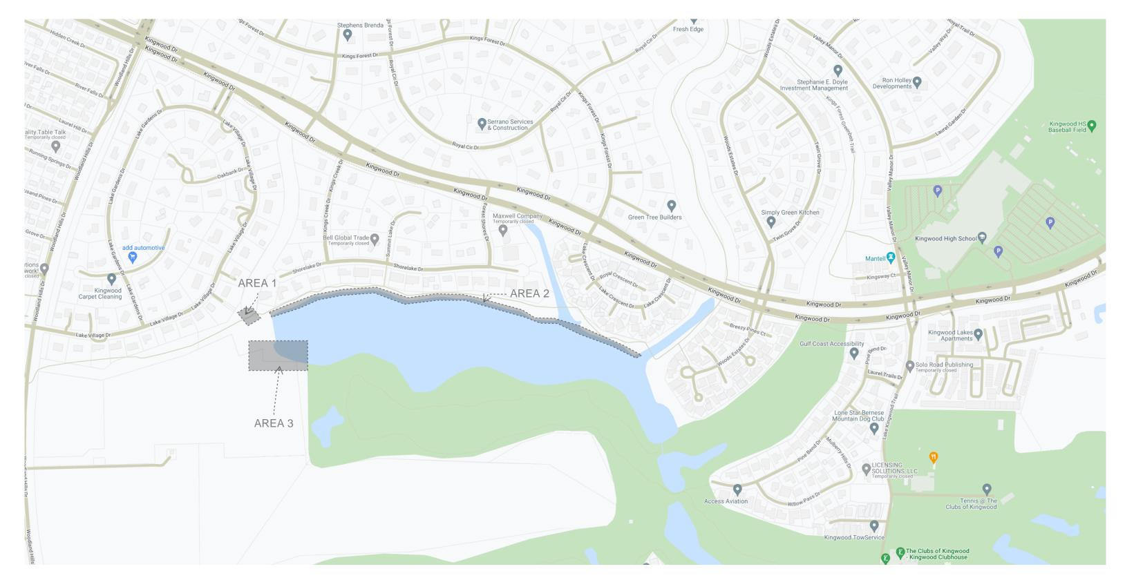
AREA 1 - BULKHEAD REPAIRS, INFILL WASHOUT BEHIND BULKHEAD, REMOVAL OF SILTATION BUIL-UP AT LAKE OUTALL AREA 2 - REPAIRS TO BULKHEAD AT WEEPS CREATING SINKHOLES, BACKFILL HOLES AREA 3 - CLEAN CANAL OF SILTATION AND GROWTH FROM BOAT RAMP OUT TO DOCK, REPLACEMENT OF DOCK, REMOVAL OF DEBRIS FROM PARKING LOT
